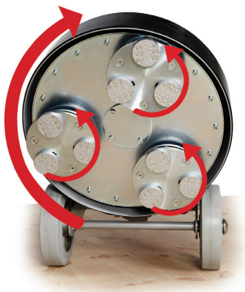
Figure 41 Illustrates the rotation of the grinding heads versus the gear barrel.
