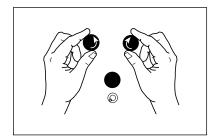
6. Observe the location of the bubble (top or bottom of the bull's-eye) and using the left-thumb rule, turn the Y axis screw to move the level bubble so that it is centered in the bull's-eye.
