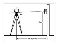
5. Measure the difference between the two marks. If they differ more than <sup>1</sup>/<sub>8</sub> inch at 100 feet (3.0 mm at 30 m), the laser needs calibrating.
