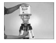
Note: When the laser is initially turned on, the out-of-level LED flashes to show that the laser needs leveling.
